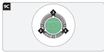
Line up the legs of the lens holder with the notches on the lamp holder and push the lens holder on.
