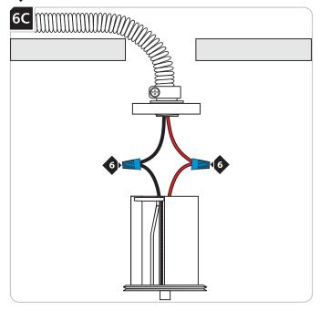
6 Connect the red and black wires in the test switch port to the same color wire in the flexible conduit using wire nuts.
