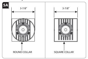
For round trims, mark a 3-7/8" diameter circle on drywall. Cut out the marked section.
