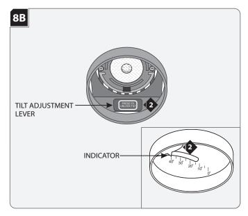
**NOTE:** Lamp housing can tilt 40° vertically. Lock intervals are 2.5° apart.
