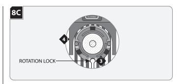
**NOTE:** Lamp housing can rotate 361° horizontally.
